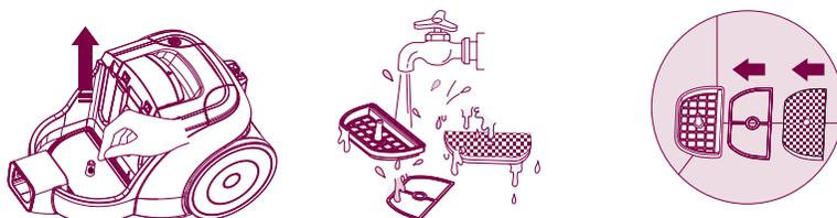
**Warning: Please check the assembling of the protection filter before using the cleaner again**
