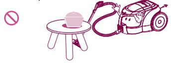
Do not use without dust tank or filters in place. Change tank frequently when picking up very fine materials such as powder.
