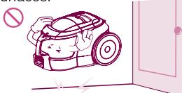
In winding the power cord, hold the plug before pressing the button of the cord reel. Do not pull the power cord beyond the red warning line, otherwise the power cord may be damaged or unable to be wound up. Pay attention to the plug in winding the cord to avoid damaging the surrounding objects.
