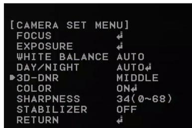
1. Select the [3D-DNR] option. If pictures are not clear due to brightness, use this function to reduce the noise of picture.
