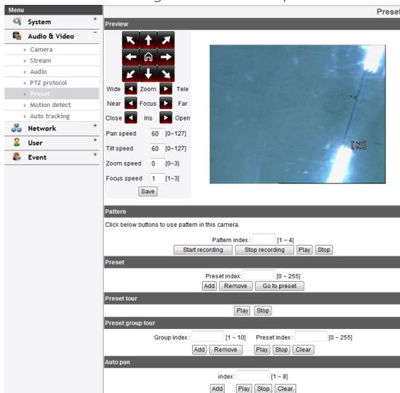
1. Move the camera to the point you want by using the arrow buttons.
