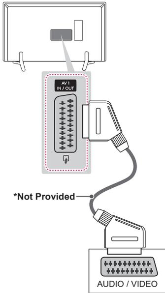
Transmits the video and audio signals from an external device to the TV set. Connect the external device and the TV set with the euro scart cable as shown.
