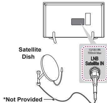
Connect the TV to a satellite dish to a satellite socket with a satellite RF cable (75 Ω).
