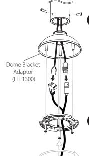
Insert the Dome Bracket Adaptor to 1.5" NPT screwthread (female) pipe or to the Wall/Ceiling/Parapet Mount Adaptor (LBK1000W/LBK1000P/LBK1000R) and tighten the three pipe screws.
