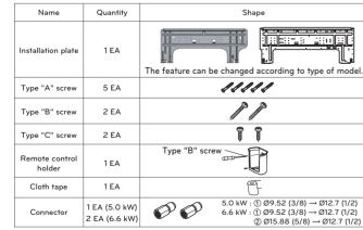
Screws for fixing panels are attached to decoration pane When Indoor unit (5.0/6.6 kW) is connected to the Multi Outdoor unit, use the connector
