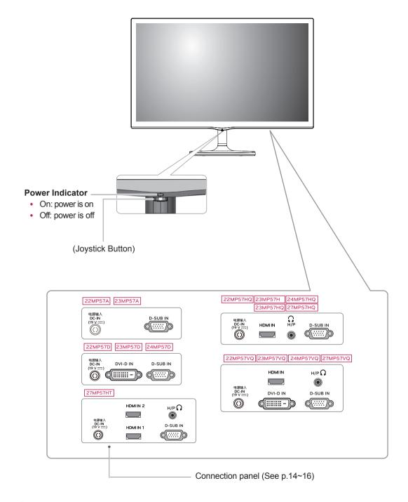
• The joystick button is located at the bottom of the monitor.
