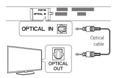
2. Set the input source to OPTICAL. Press **F** button repeatedly until the function is selected.
