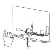
Do not use a sharp object when you detached the cable cover. This could damage the cable or the cabinet.
