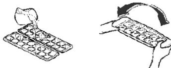
Do not use sharp tool to remove ice tray, otherwise you may puncture the evaporator resulting gas leakage thus non performance of refrigerator.
