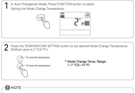
The Mode Change Temperature is the difference of temperature when from cooling mode to heating mode or from heating mode to cooling mode.
