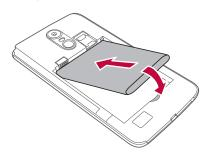
3 To replace the cover onto the device, align the back cover over the battery compartment and press it down until it clicks into place.
