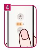
Press the LEVEL button for a short time and select the strength.
