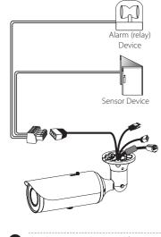
The Photo MOS Relay is rated for . 100 mA at DC 20 V or 100 mA at AC 28 V.
