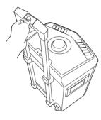
3. Release the lock button to lock the handle in place.
