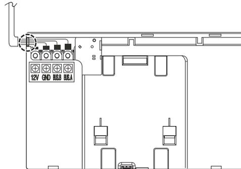
Fix it by using screw provided at the lower part tightly after wet it up the bracket.
