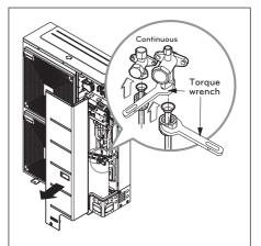
\* When tighten the pipe, hold the haxagonal body.
