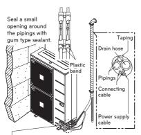
Trap is required to prevent water from entering into electrical parts.
