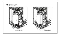
When connecting in a downward direction, knock out the knock-out hole of the base pan. (refer to figure 2)
