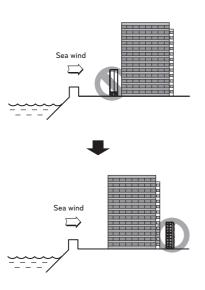
In case, to install the outdoor unit on the seaside, set up a windbreak not to be exposed to the sea wind.
