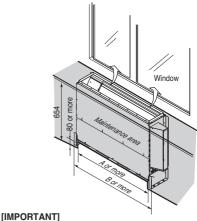
Leave sufficient clearance for air inlet and maintenance.
