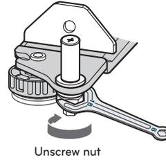
(2) Use the narrower side of the spanner to turn the adjustment hinge pin (↻) clockwise or (↺) counterclockwise, and adjust the gap difference between the fridge and the freezer door.
