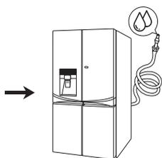
3 Connecting the water supply and water line
