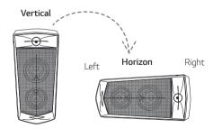
On the horizon mode, you can hear the stereo sound and on the vertical mode, the sound transforms into a mono signal.
