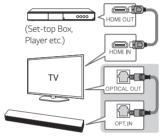
2 Set the input source by pressing **OPTICAL** on the remote control.
