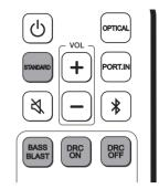
STANDARD/BASS BLAST : Selects the sound effect. DRC ON/OFF : Makes comfortable sound at Dolby Digital.
