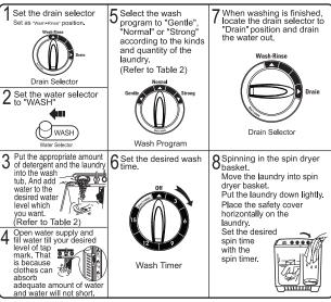
Program for test accordance in conformity with SASO 2692:2013 and SASO 2693:2007 setting Wash 35 min (Water Level: H level) Rinse 5 min. / Spin 10min (2times, 5min/1time) Water (Hot 32 Litres / Cold 42 Litres)
