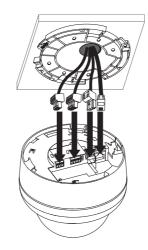
4. Assemble the camera and mounting bracket after align the front part of the camera and mounting bracket. Connect the unit by following step 1 and 2.
