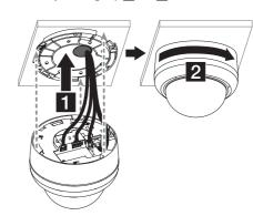
Be careful of sharp edge after removing the cap of cable conduit.
