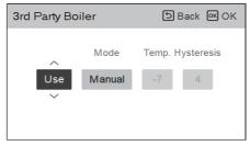
If the mode of this function is set to "Manual", you can set temperature of the boiler and hysteresis, respectively.
