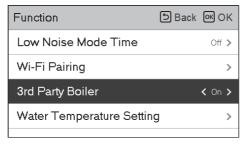
On/off mode of this option are opened by pushing "<" or ">" button simply and easily.
