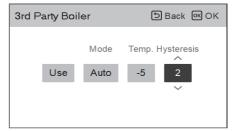
AS shown above, After every setting is completed in installer mode, 3rd party boiler option is activated in function list.
