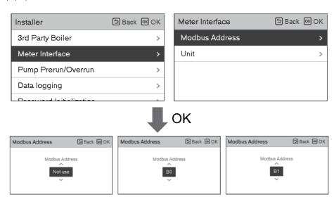
There are 2 options, modbus address and unit, in this function. Activating the modbus address option, you choose one address(B0 or B1) or don't use. Then, you set the port and specification in range of 0000.0~9999.9[pulse/kW] as shown in the figure below.
