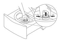
Open the cap and remove lint and then wash out.
