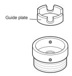
Push the adapter onto the end of the tap so that the rubber seal forms a watertight connection. Tighten the four fixing screws and the adapter ring plate.
