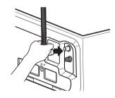
3 Adjust the hose clip in place to prevent leaking.
