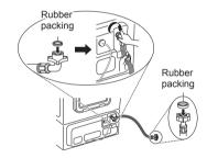
3 Connect the additionally provided water supply hose of the front-loading washing machine to the water supply hose connector and water faucet.
