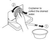
Remove any extraneous matter from the pump filter.
