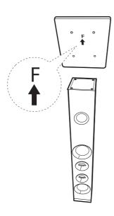
3. Tighten up with supplied screws.
