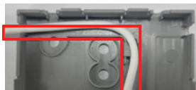
Reference. the bent cable shape
