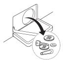
▲ After cleaning, refit the pump filter and insert the drain tube plug.
