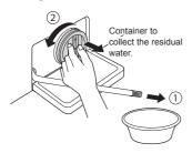
3 Remove any extraneous matter from the pump filter and cavity.
