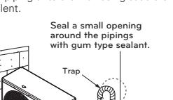
In cases where the outdoor unit is installed below the indoor unit perform the following.
