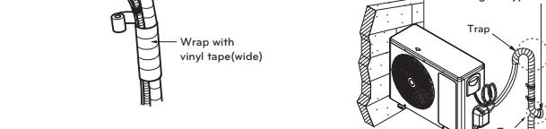
In cases where the outdoor unit is installed below the indoor unit perform the following.
