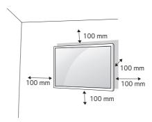
To install your monitor on a wall, attach a wall mounting bracket (optional part) to the back of the monitor. Make sure that the wall mounting bracket is securely fixed to the monitor and to the wall.
