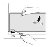
Insert a small flat screw driver into the hole of the movable pin. Slide the pin to the right and remove the mini table.
