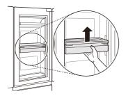
2 To lower moving basket, press up to release the levers at the side of the basket and lower the basket until it clicks into place.
