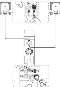
2. Connect the wireless receiver and the rear speakers (left, right) with the speaker cables.
