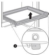
4 To refit, hook the drawer support on the rails located on both side and press it down until you hear snap sound.
