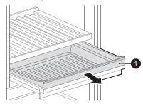
**2** Lift the drawer straight up and out of the frame.
