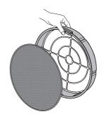
5. Assemble the filters as reverse way after cleaning and filter replacement, and insert the filters as the filter handles are located at the top of the product.
