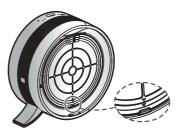
5. Mount the filter by matching the rear panel to the bottom part.
