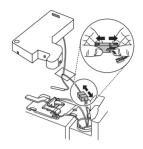
3 Rotate the hinge lever counterclockwise. Lift the top hinge free of the hinge lever latch.
