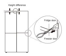
Loosen the keeper nut by rotating it 1 counterclockwise using a 19 mm spanner.
