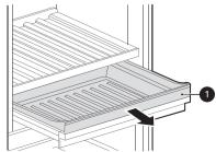
**2** Lift the drawer straight up and out of the frame.
