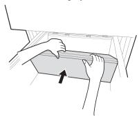
7 Insert the supplied hole cover into the groove at the bottom of the drawer.
