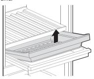
3 Keeping both levers 2 pressed, lift the drawer support slightly and remove it from the rail.
