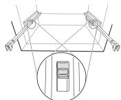
5 Angle the drawer into the frame and set it in place.
