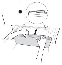
3 Hold the middle of the cover and lift it slightly into the groove.
