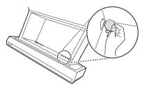
2 Raise the back section of the folded cover and rest it on the guide a at the rear of the drawer.
