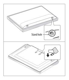
Screw length from outer surface of back cover should be under 8 mm. (Only 24/28LV76\*\*)
