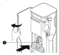
2 Open the right door and insert the combination tool **2**, the crevice tool **3** and the cleaning brush **4** for storage.
