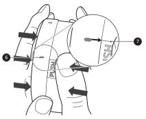
8 Push and insert the exhaust filter cover 3 into the exhaust filter 1 and rotate it to reassemble it and prevent it from falling out.
