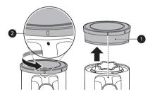
**3** Grip the exhaust filter cover **③** and the exhaust filter **①** using both hands and rotate the exhaust filter cover while pressing the **PUSH** button in order to separate it from the exhaust filter.
