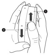
**9** Insert the dried pre-filter and rotate the exhaust filter to the locked position **(3)** to reassemble it on the product body.
