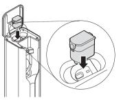
**3** Press the battery down into the compartment.
