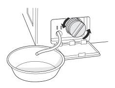
Clean the pump filter and opening.
