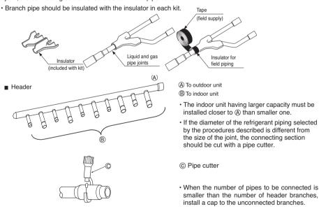
• When the number of indoor units to be connected to the branch pipes is less than the number of branch pipes available for connection then cap pipes should be fitted to the surplus branches.
