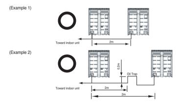
· When connecting the pipes between the outdoor units, the accumulation of oil in the slave outdoor unit should be avoided. Otherwise, the unit may not operate properly.
