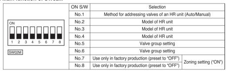
1) Selection of the method for addressing valves of an HR unit (Auto/Manual)
