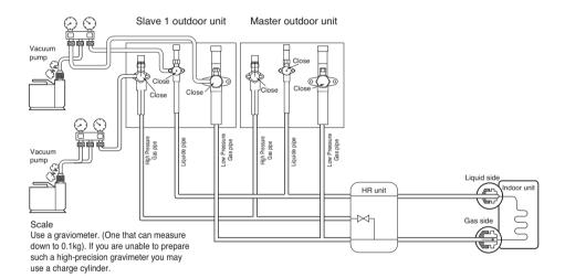
Note: Always add an appropriate amount of refrigerant. (For the refrigerant additional charge) Too much or too little refrigerant will cause trouble. To use the Vacuum Mode
