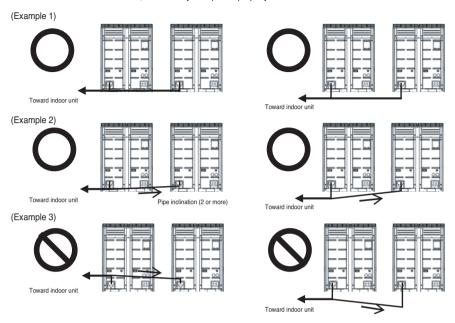
• Apply Oil Trap as shown below when the length of the pipe between the outdoor units is more than 2m. Otherwise, the unit may not operate properly.
