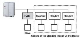
\* FAU : Fresh Air Intake Unit Standard: Standard Indoor Unit
