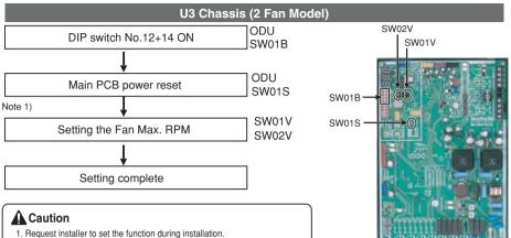
In case the function is not used, set the DIP switch OFF and reset the power.
