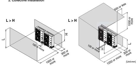
⊃ Obstacle height of discharge side is lower than the unit
