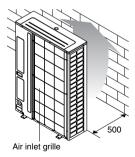
Turn the air outlet side toward the building's wall, fence or windbreak screen.
