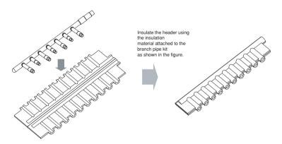
• Joints between branch and pipe should be sealed with the tape included in each kit.
