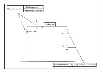
Pay special attention to the place, such as a basement, etc. where refrigerant can be present, since refrigerant is heavier than air.
