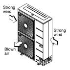
Set the outlet side at a right angle to the direction of the wind.
