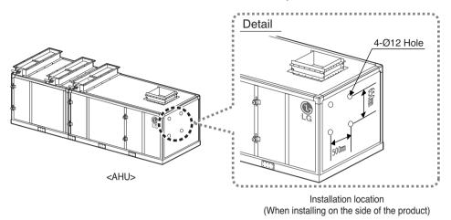
2. Check location of the hole on the rear side of CONTROL KIT and check whether accessories exist for the installation.
