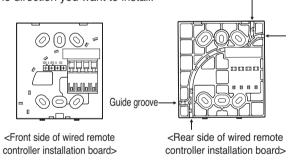
3. After locating the wired remote controller installation board at the location you want to install, tighten the screw to firmly fixate it. (If there is a burial box, install the wired remote controller installation board to fit the burial box.)
