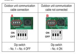
· Adjust Rotary switch of the part connected to Outdoor unit communication cable.
