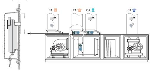
■ During the outdoor installation, the protection cover must be installed on the sensor. If not installed, the rain water may enter inside the sensor, and cause disorders.
