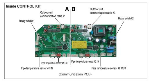
· Adjust Dip switch depending on the connection of Outdoor unit communication cable
