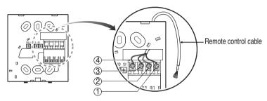
2. After fixating the cable on the guide groove, attach the installation board of the wired remote controller to the location you want.
