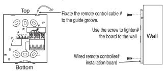
4. After fixating the top part of the remote controller to the wired remote controller installation board. press the bottom part to assemble to the board. When separating the remote controller from the board, use the driver as shown in the right picture to insert the driver into the hole marked with the arrow and pull the driver to separate the remote controller.
