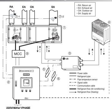
Installation components No. Name Remarks 1 Air Handling Unit (2) CONTROL KIT PRCKD20E / PRCKD40E EXPANSION KIT (3) PATX13A0E/20A0E/25A0E/35A0E Outdoor unit Multi V **(4)** Pipe temperature sensor IN Sensor: Ø5, Length: 10m, Cable color: Black (5) (6) Pipe temperature sensor OUT Sensor: Ø7, Length: 10m, Cable color: Red Temperature sensor RA -50~50°C/ AC 24V / DC 0~10V (7)-1(7)-2Temperature sensor SA -50~50°C/ AC 24V / DC 0~10V Return Fan 8-1 Supply Fan (8)-2 MCC 9 MCC
