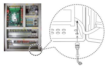
3. Classify the IN/OUT of the pipe temperature sensor, and connect to the connector on the communication PCB.
