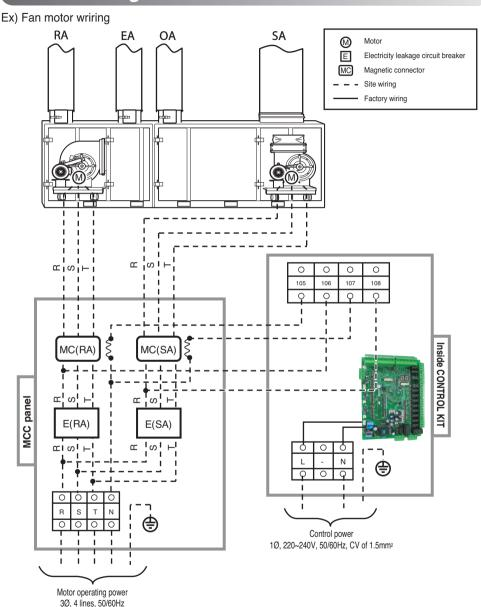
Select and use the standard product (Power cable/Circuit breaker/Magnetic contactor)
