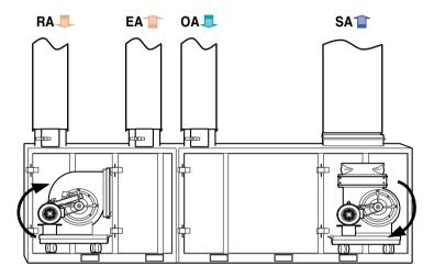
2. If the damper actuator is installed as an option, check whether the dampers are configured to open as follow 2 minuts after the power is connected.
