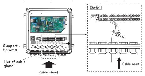
4. For the wired remote controller wire and outdoor unit communication wire, remove the coating at the end of the wire to connect and use the ring type (Ø3) to connect to the terminal block.
