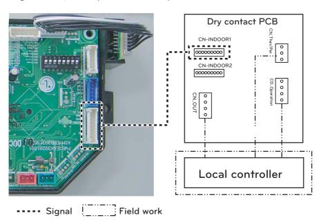
2. Using cable, connect the dry contact to main PCB. For more information, please refer to dry contact installation manual.
