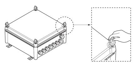
2. Drill 4 holes on correct position and fix the Control Kit box securely with 4 screws(Field supply) through the provided holes Ø4.5 mm(Reference the length of the holes Ø4.5)
