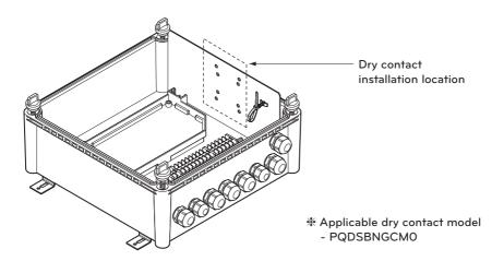
1. Using screw(4EA), fix the dry contact on the side panel.
