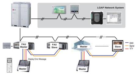
In case of connecting with standard indoor unit and Fresh Intake Unit, separate Fresh Air Intake Unit with standard units.
