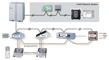
It is possible to control N indoor units by wired remote controller M units. (M+N≤17 Units) Set only one indoor unit to Master, set the others to Slave. Set only one wired remote controller to Master, set the others to Slave. Other than those, it is same with the Group Control 1.
