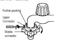
Turn the middle connector not to have water leaked. 3 Connect the water supply hose to the middle connector, pushing the plate down.
