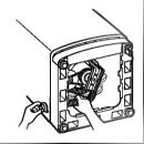
Fasten the set screw to secure the drain hose joint.
