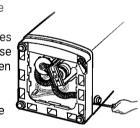
2 Change the direction of the drain hose to the hole of the opposite side.
