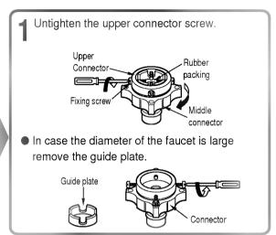
Push the upper connector up till the rubber packing is in tight contact with the faucet. Then tighten the 4 screws.
