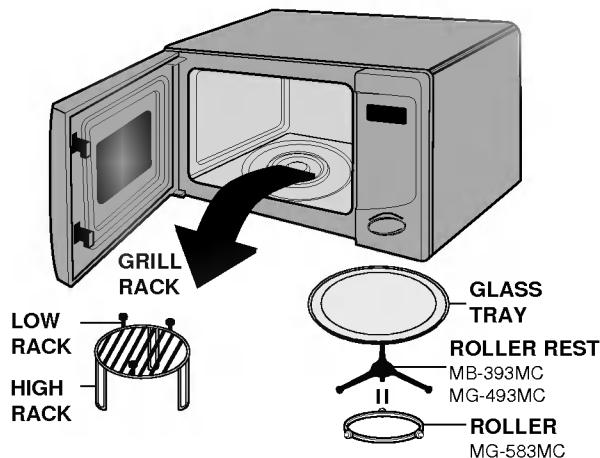
2. Place your oven on a flat, level surface but make sure there is at least **10 cm** of space on the top, rear and sides so there is air flow for ventilation. Exhaust outlets are located in the back and side of your oven. Blocking the outlet can damage your oven. THIS OVEN IS DESIGNED FOR BUILDING IN. (Not over a heat source)
