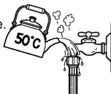
2 Submerge the separated hose in hot water (about 50°C).
