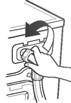
4 Pull out the filter with a tool or by hand and clean it using a toothbrush.
